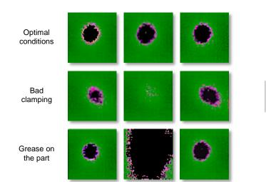
▶ Inspection post-manufacturing in DMD (parameter : surface of the weld pool)
