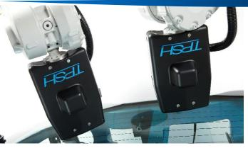
We have developed a very high speed (4 to 12m/s) robotized confocal measurement system allowing in-line quality control of 100% of the production.
